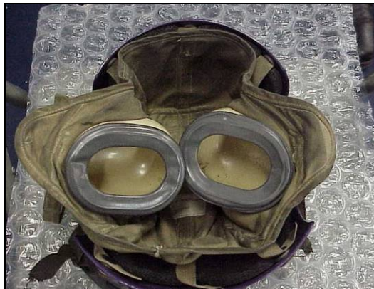
Figure 14: Survey Subject's Cranial in Poor Condition (Note Hard-Creased Earcup Cushions, Missing Earcup Foam Inserts, and Dirty Cloth)
