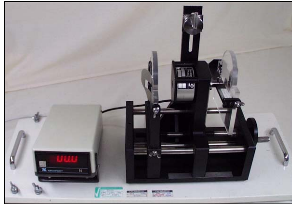
Figure 8: Inspec Laboratories, Ltd. Rig to Measure Earmuff Headband Clamping Force
