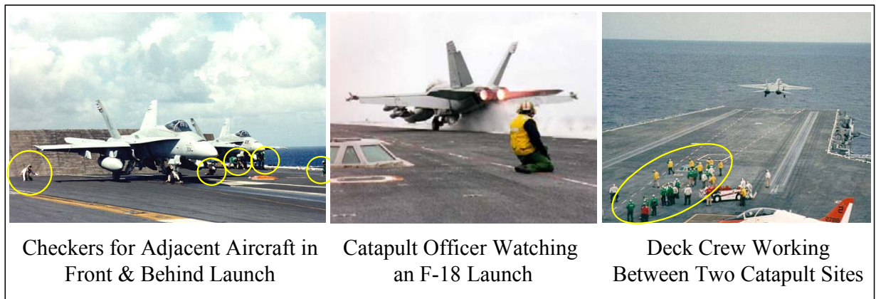
Figure 6: Photographs of Deck Crews at Work in Close Proximity to Jet Noise
